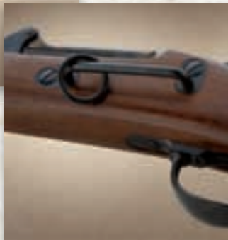
The Springfield Trapdoor Carbine is fitted with a sliding ring and bar, which allowed a cavalryman to carry it clipped to his carbine sling.
