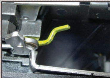
Sear Deactivation Lever Disassemble the Handgun without Pulling Trigger
