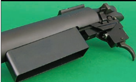
The metal box magazine is attached to the receiver, a good idea when employing a blind magazine.
