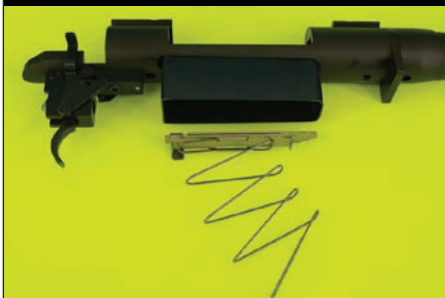
A coil, rather than a flat spring, powers the follower in all ATR models.
