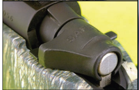
If inadvertently de-cocked (top photo), the flange on the bolt shroud precludes the bolt from being pushed home (bottom photo).
