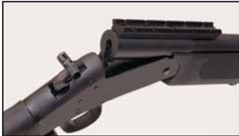
308 Win. and 223 Rem. bull barrels are equipped with Weaver-type scope mount and hammer extension.
