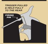
All NEF and H&R single shot firearms incorporate a special safety feature – a transfer bar system that prevents the gun from being fired unless the hammer is fully cocked and the trigger pulled and held completely to the rear.
