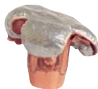
30 cal. 150 gr. 2473 FPS Retained 141 gr. 94% Wt. Ret. .692" Expanded
