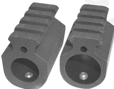
A great addition to both standard and bull barrels, these gas blocks are machined from solid aluminum extrusion. Cut with standard picatinny rails, they will accept all picatinny standard hardware including detachable A-Frame style front sight bases and globe sights. *Please specify the diameter when ordering; (.728") Standard or (.928") Bull diameters.*
