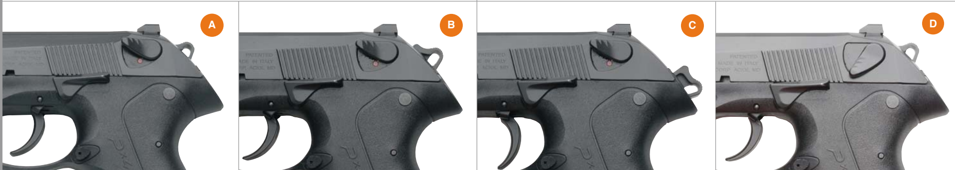
F MODELS. SAFETY DISENGAGED: A)HAMMER DE-COCKED B)HALF-COCKED HAMMER C)COCKED HAMMER
