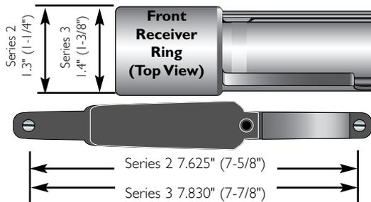
**Series 2 (93, 94, 95, 96)** — 1-1/4" front receiver ring and 7-5/8" center to center on the trigger guard screws. This series includes most Model 93, 94, 95, 96 rifles and carbines.
