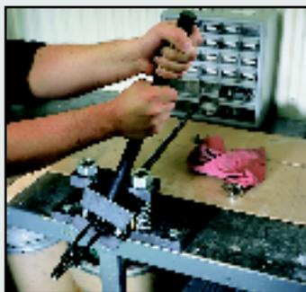
The double-ended Savage Barrel Nut Wrench fits both early and late model nuts on the 110 and 10 series rifles, and features two 1/2" square drive holes for a swing bar or torque wrench. The Barrel Vise provides plenty of holding force to securely clamp your barrel for removal or installation. The Vise includes two pre-drilled oak blocks, 1" and 3/4", and a solid block for custom drilling.
