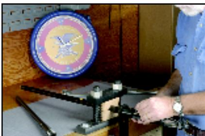
4. The new barrel is clamped in the vise, the receiver is screwed onto the barrel, and the headspace gage is inserted into the chamber.
