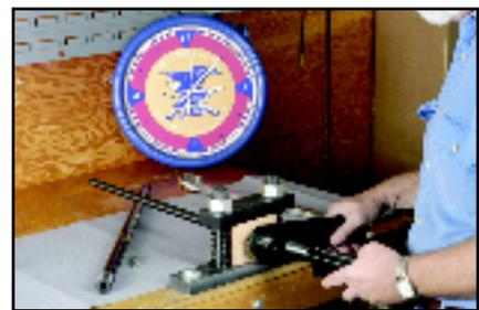
3. With the barrel nut loosened, the receiver is unscrewed from the barrel.
