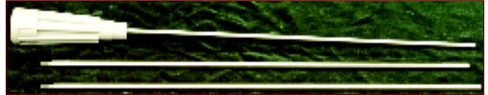
All the features shooters demand in a cleaning rod, at an affordable price. Fouling and abrasive particles cannot imbed in the hard, stainless steel shafts. The tough, chemical-resistant handle features a self-lubricating bearing for smooth rod rotation while cleaning. Pistol and rifle rods have 8-32 female threads (except 17 caliber, 5-40 thread). Shotgun rods accept standard 5/16"-27 threaded accessories.
