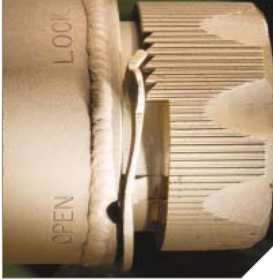
SureFire's suppressor uses an ingenious "Fast Attach" lock ring to secure the unit to a special flash hider.
