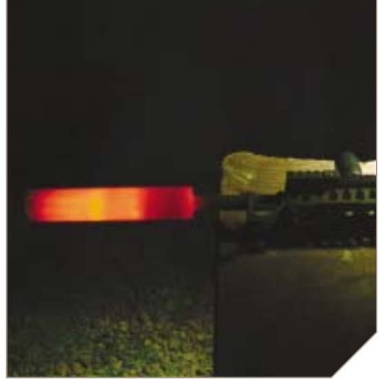
The suppressor glows bright orange after 1,500 rounds—that's 50 30-round mags—fired full-auto.
