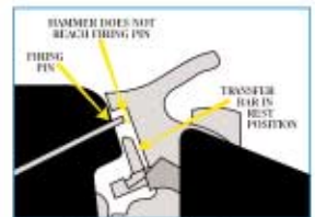
The transfer bar mechanism prevents the hammer from striking the firing pin unless it has been cocked and the trigger pulled rearward.
