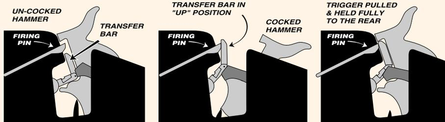
All NEF and H&R single shot firearms incorporate a special safety feature – a transfer bar system that prevents the gun from being fired unless the hammer is fully cocked and the trigger pulled and held completely to the rear.
