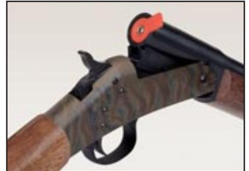
The primer is held in place by a special, patented, reusable primer carrier, which also serves as a visual indicator that the rifle is primed (Both Models).
