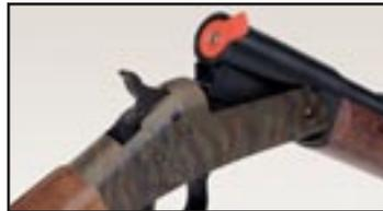
The primer is held in place by a special, patented, reusable primer carrier, which also serves as a visual indicator that the rifle is primed (Both Models).
