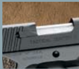
Tactical pistols have the new, innovative Kimber Tactical Extractor with loaded chamber indicator feature.
