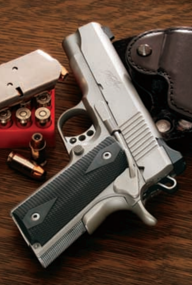
Compact and Pro Carry models have 4-inch bull barrels fitted directly to the slide without a bushing.
