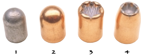
The basic manufacturing stages of Gold Dot bullets.
